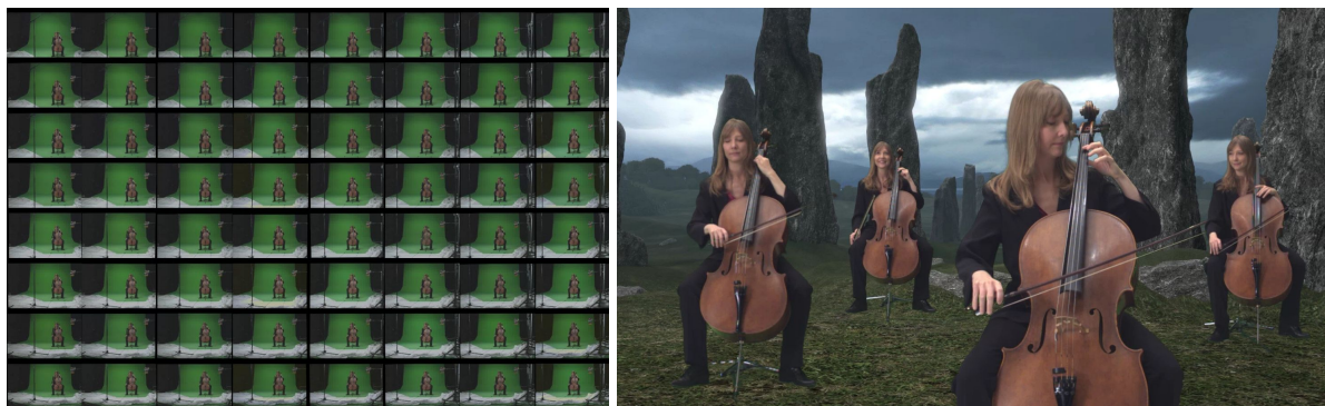
Left: light field frame containing the 64 camera views Right: snapshot from the 'Unfolding 2.0' holographic output
